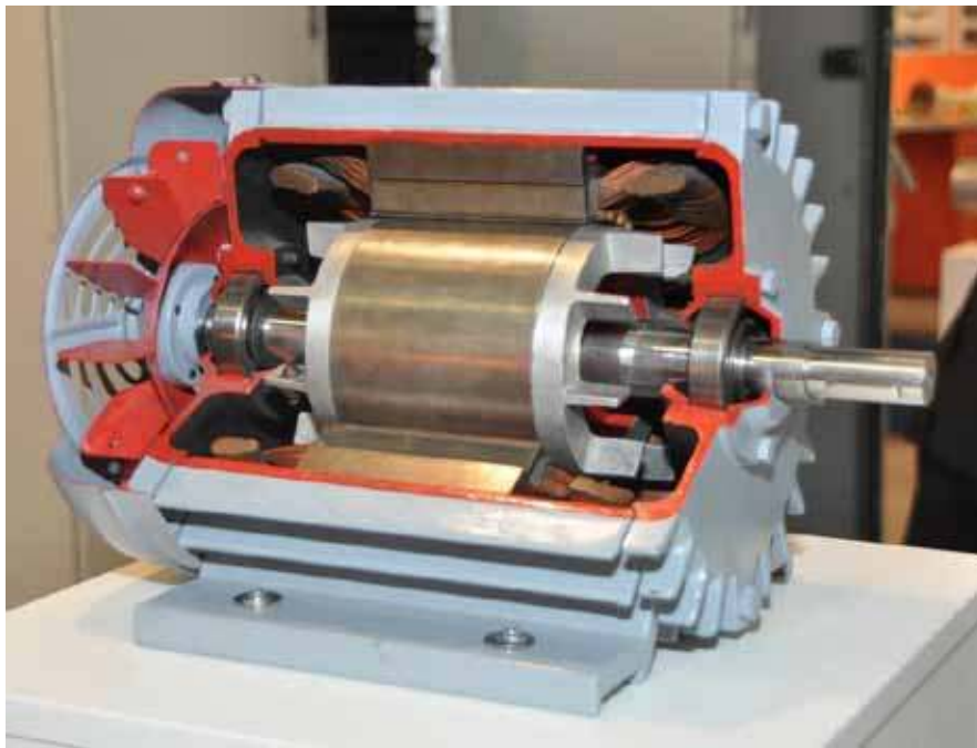
รูปที่ 1-24 Cutaway view through stator of induction motor
